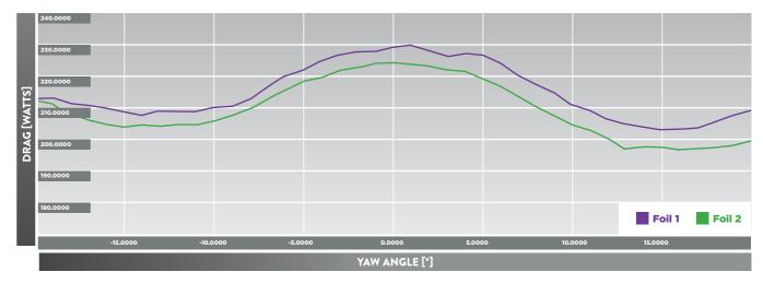
Drag Power [W] vs. Yaw Angle [°] at vapp = 45 km/h (Bike with moving legs / Shimano Dura Ace Di2 / Zipp 404 / 1 Bottle on Downtube)
